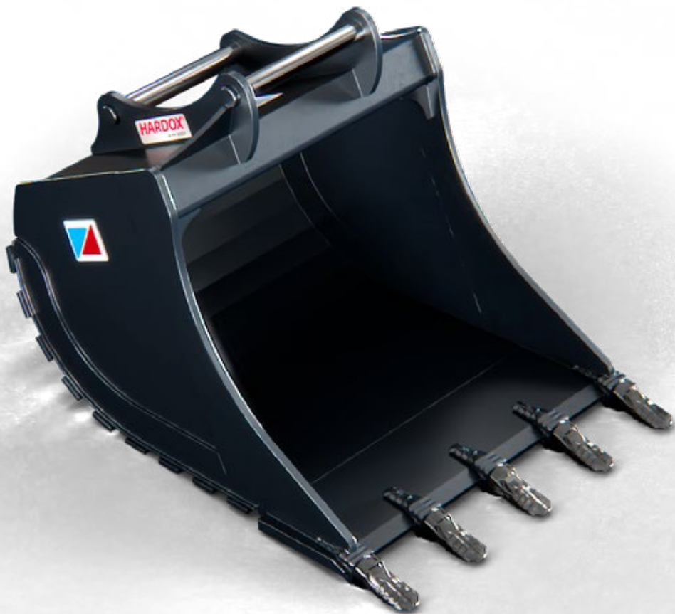
DSX heavy duty digging bucket in the Nordic profile for excavators from 14 to 40 t. Body in Hardox® 450 steel for rocky ground, abrasive material, demolition and quarries.
